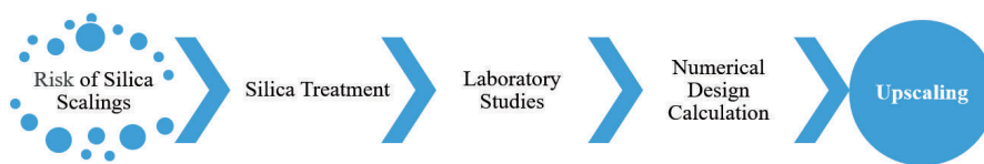
Fig. 4 Flow chart summarizing the problem-solving approach in the BrineMine project. Based on the challenge of silica fouling, a treatment strategy was developed in the laboratory. This approach was upscaled first using a numerical design calculation. The simulation results were subsequently reproduced in a technical center leading to the construction of a 1st generation prototype.
